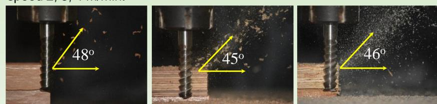
The flow area was different among the wood-based materials due to the difference in their structures. Left to right: WPC, LVL, OSB. Feed speed 3 m/min, 75° helix angle.
