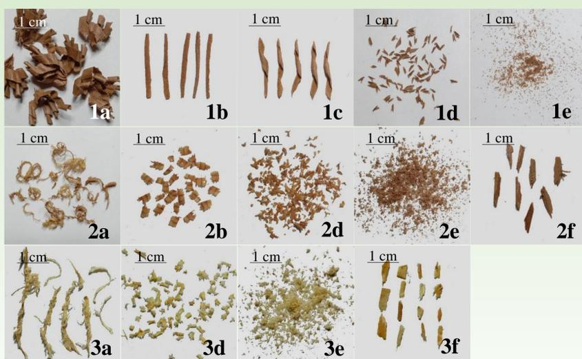
The chip shapes generated in cutting WPC (1), LVL (2), and OSB (3) were classified as continuous chip (a), flow chip (b), spiral chip (c), thin chip (d), granule/powder chip (e), and splinter chip (f).
