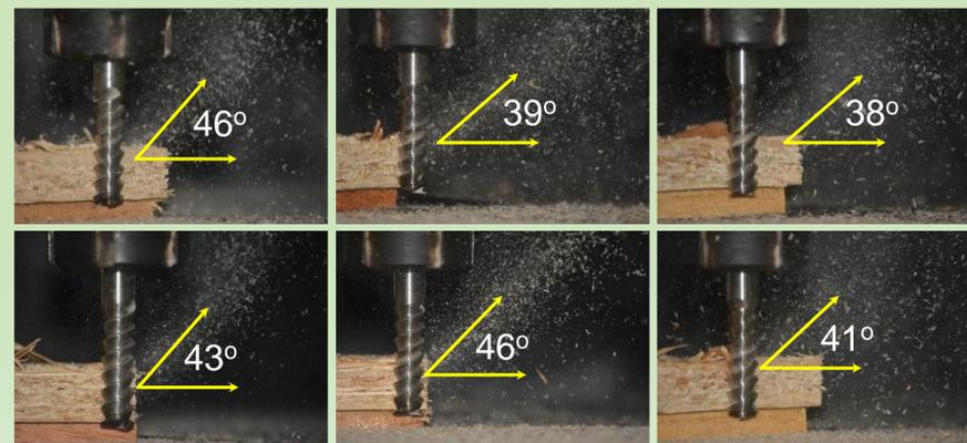
The flow area in up-milling (upper) was larger than in down-milling (lower). Increasing of feed speed resulted in a larger area of flow and was observed to produce a higher speed during cutting. Left to right: feed speed 2, 3, 4 m/min.
