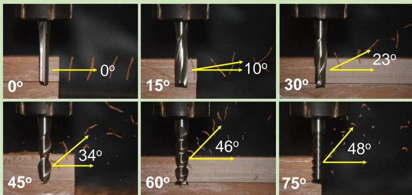
With increasing the helix angle, the chip flow angle to the tangential direction became larger, the sector area of the chip flow became smaller, and the speed of flow was observed to be lower
